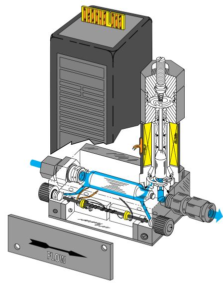
Figure 3: Heated tube mass flow controller
