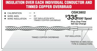
SINGLE PAIR OF SOLID TYPE K TC WIRE WITH FEP
