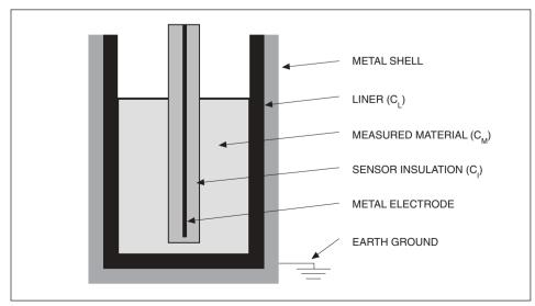
Figure 1 - Capacitive Measurement Path In Lined Metal Vessel
