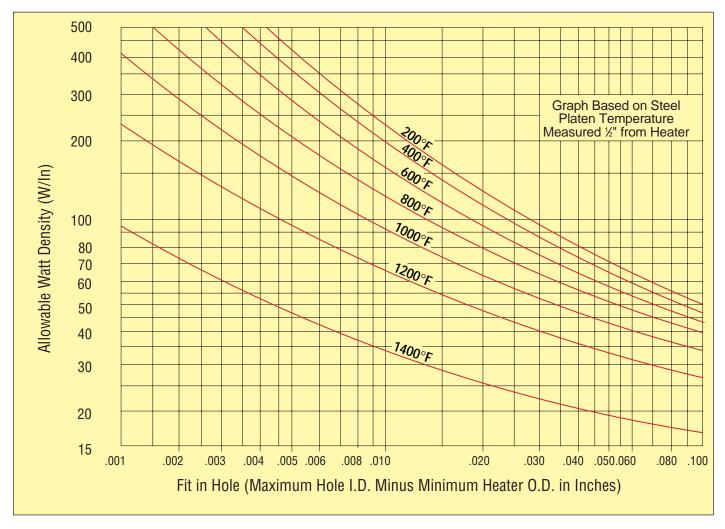
FIGURE D-1 Allowable Watt density vs platen temperature for various fits using OMEGALUX® Type CIR cartridge elements.
